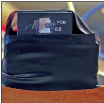
■ FIGURE 4. Close-up of laser mounted in showerhead. The showerhead articulates in a ball and socket fashion. This particular model of showerhead had a gasket which permitted a press fit of the laser unit without further modification. Other heads may require glue or creation of a sleeve around the laser to allow a press fit. Wires follow the water path.
